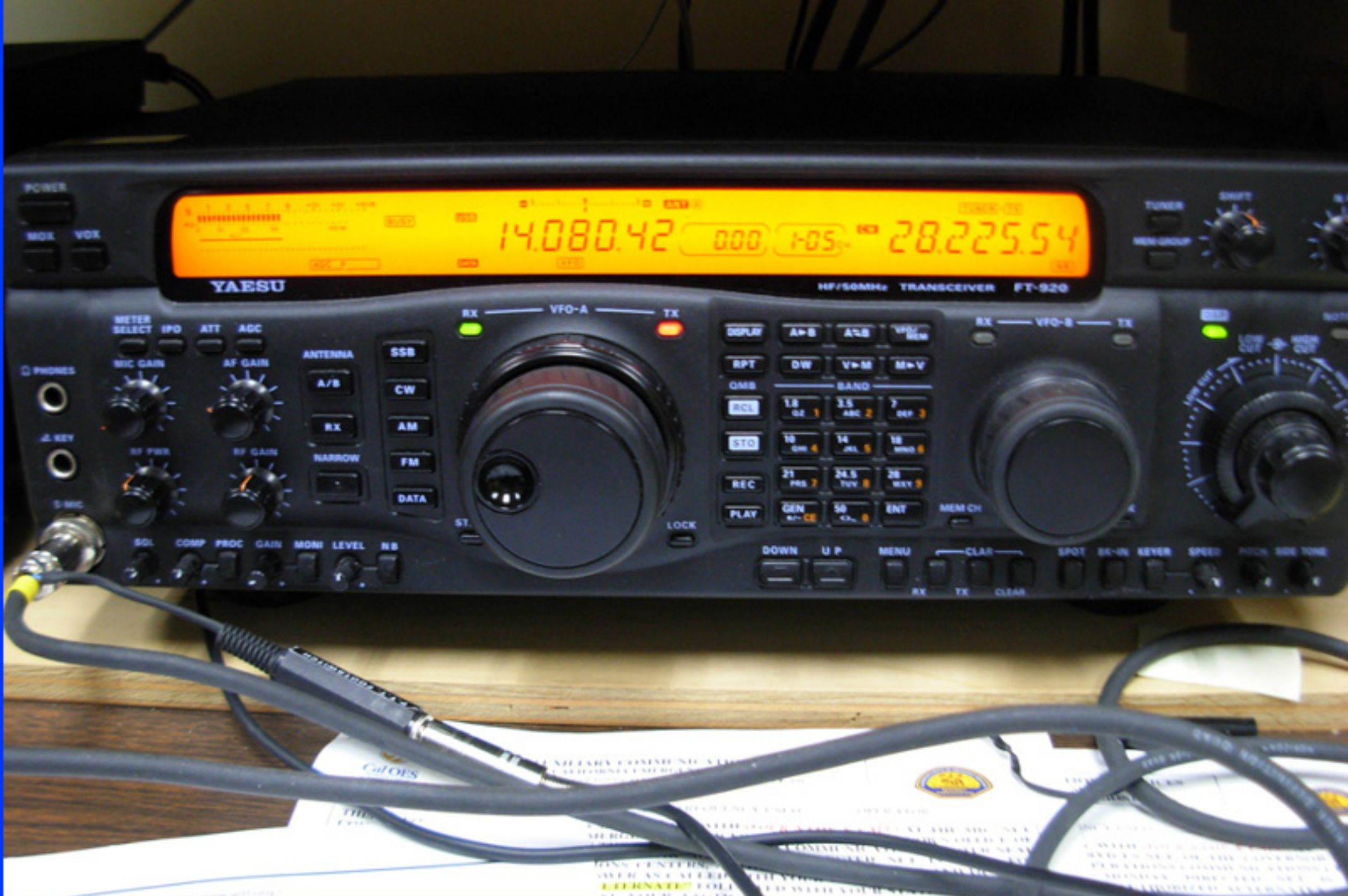
Otech's ECC Yaesu FT920 HF xcvr was used for digital modes PSK31 & RTTY on 20m
